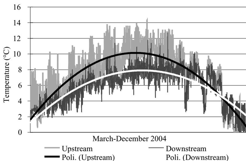
Fig. 2 - Temperatures (°C) recorded from March to December 2004 in a station upstream (NB7) and downstream (NB8) of the turbinated water release point at Cogolo-Pont plant.
