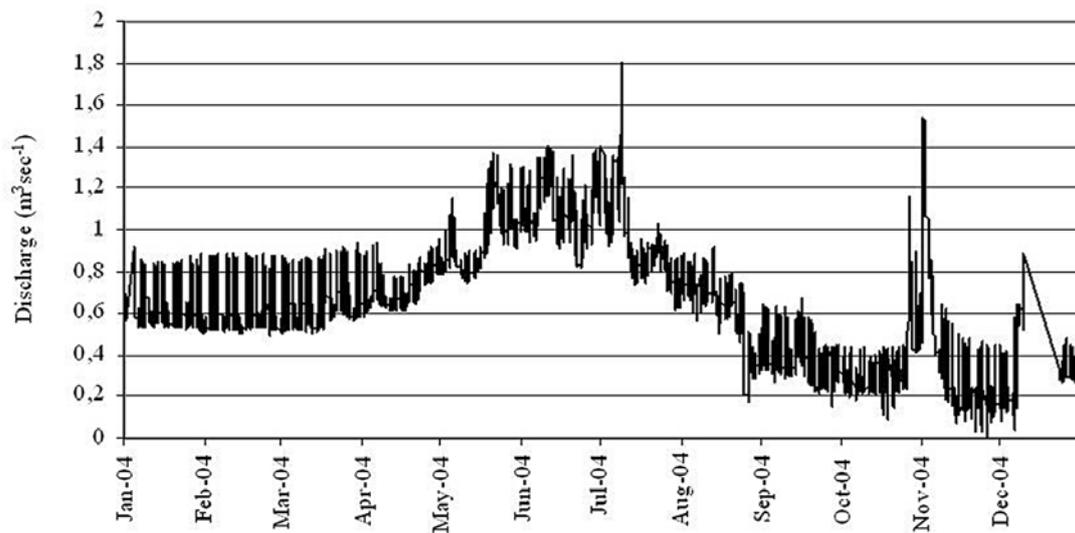
Fig. 3 - Discharge ( $\text{m}^3 \text{sec}^{-1}$ ) during hydropeaking regime recorded at the Service for Hydraulic Works Hydrological monitoring stations located at Noce Bianco stream, downstream from Cogolo-Pont hydropower station
