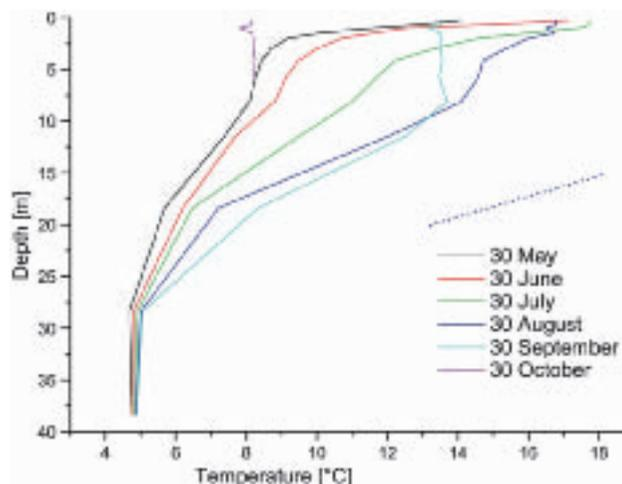
Fig. 5 - Seasonal evolution of the vertical temperature profiles at chain D (dotted line: thermocline conventional slope).
