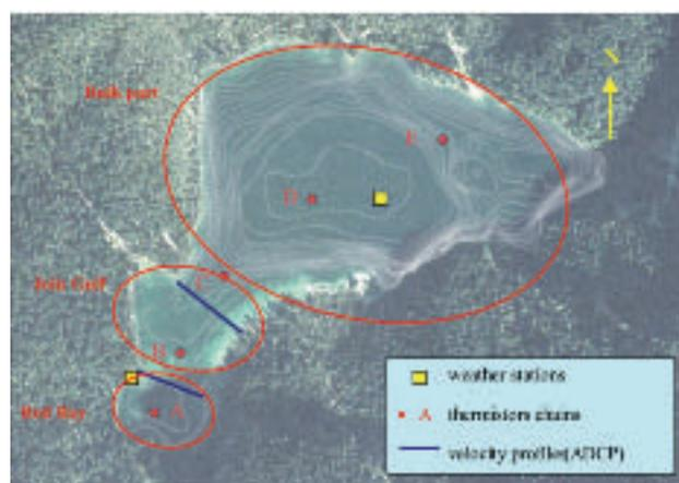
Fig. 2 - Bathymetry of Lake Tovel and location of measurement points: the circles defines the three sub-zone.
