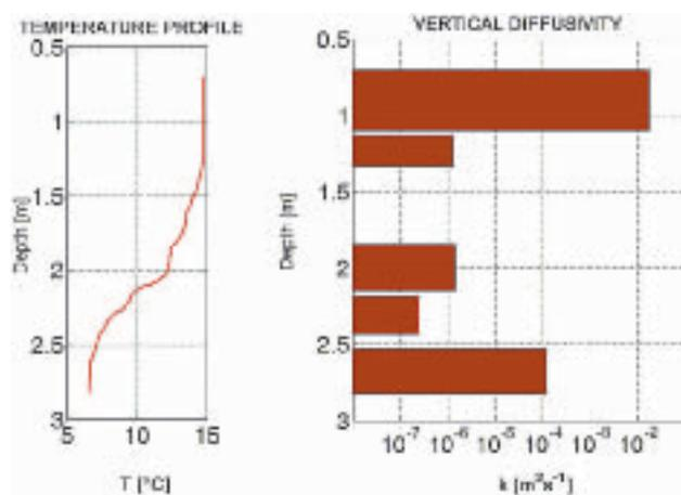
Fig. 13 - Temperature profile collected through the SCAMP profiler in the Red Bay on August 31<sup>st</sup> 2004 (left) and the vertical diffusivity (right).
