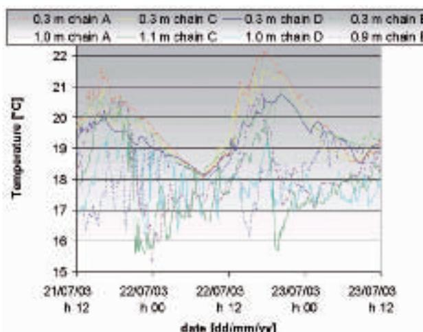
Fig. 7 - Temperature data collected near the surface and 1 m below at the thermal chains A, C, D, E. In the first windy day a strong fluctuation is detected in the evening, whose intensity decreases during the night and in the following sunny day (the black line shows the damping of the seiches).
